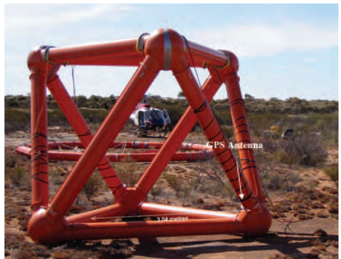
Fig. 3. ZTEM and AirMt base station sensor.
